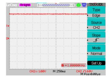
Press the front panel ACQUIRE button and note the sample rate. For the model 112 using a 250ms/div timebase this will be 1.000KSa/s.
