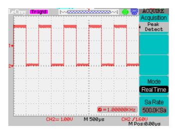
Now press the Acquisition button to select Average and allow the scope to run for a few seconds. Again note the noise levels on the signal.
