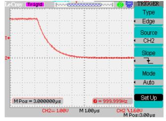
Push in the Position knob to see the trigger point revert to the center of the screen.
