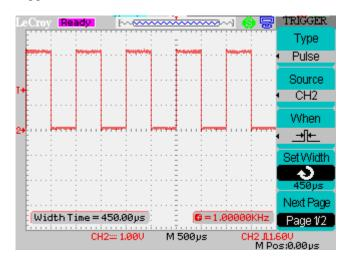
The positive pulse width for a 1kHz square wave is 500us. The Set Width control can be used to determine if we trigger on this pulse or not. As an experiment select one of the other options in the When menu and investigate the effect of changing the width setting. The Type menu also provides additional types of trigger. Operation of these trigger modes is described in more detail in the WaveAce operator's manual.
