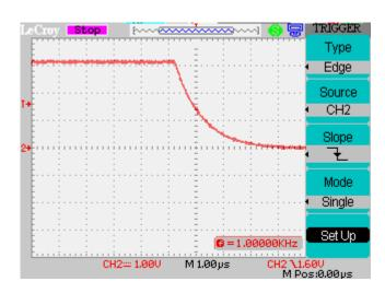
The scope should now trigger. The RUN/STOP button has changed to red and the marker displays Stop. If the edge displayed does not look like the above press RUN/STOP once more to capture a clean edge.
