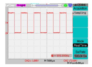
Now press the Acquisition button and Peak Detect is displayed. Allow the scope to run for several seconds. Note the level of noise on the signal.
