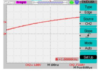
Change the timebase to 10 us/div and repeat Step 8. Note that now there is no change in the sampling rate. Equ Time mode is only useful on the faster timebases.
