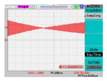
In the TRIG MENU change the trigger slope back to positive or negative edge triggering and the signal is correctly represented on the scope display.
