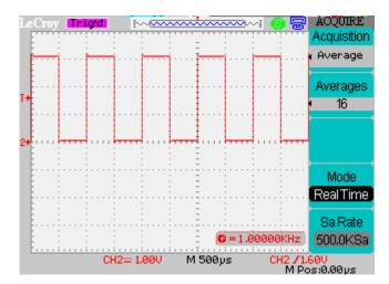
A sampling acquisition samples the waveform at uniform time intervals. A rapid variation in the signal such as a narrow pulse may therefore be missed. In Peak Detect the highest and lowest values in the signal are recorded so allowing even narrow pulses to be captured. Averaging is useful to reduce random noise. When using averaging you can also select the number of acquisitions to average. Higher values will give more noise reduction but the averaging will take longer.
