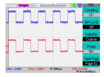
Expand the traces to full the screen by adjusting each channel's voltage and position knobs.
