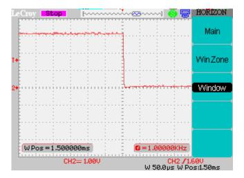
Select Main in the menu to display the original waveform and in the TRIG MENU set the mode to Auto.
