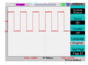
Press the Language function to change to a different language. When a button with multiple selections is pressed a small pop-up box appears alongside the button. While this pop-up is displayed the green LED above the front panel Intensity/Adjust knob is also illuminated. This knob functions as an Adjust knob and can be used to scroll through the available selections. When the LED goes out the knob reverts to its normal function.
