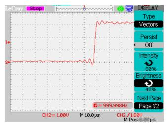
It is very important to understand that a digital oscilloscope, samples the data into discrete data points.
