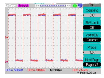
Press DISPLAY and select page 2. Press Format to select XY. CH1 is now plotted against CH2 instead of both waveforms being plotted against time. Both waveforms are the same here so the resulting XY plot is not very interesting. In a real situation XY plots can provide significant additional information. Dot mode is always used for XY plots so turning on Persistence (DISPLAY menu page 1) is often beneficial.
