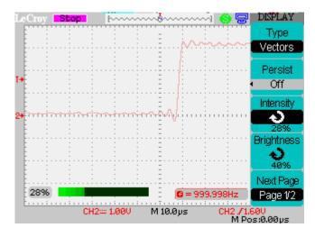
Select Brightness and now the front panel Intensity/Adjust knob controls the grid intensity. An onscreen bar is momentarily displayed when adjusting.
