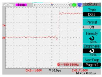
Change back to Vectors and observe that the sample points are joined by lines. In most cases this is the best configuration.
