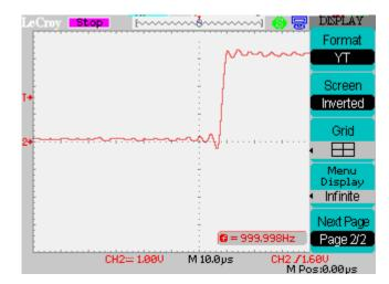
Press the Menu display to control menu operation. Selecting a value other than Infinite will result in the menu automatically disappearing after the specified time.
