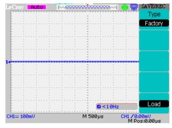
At any time the menu on the right-hand side of the screen can be removed/restored by pressing the front panel MENU ON/OFF button.
