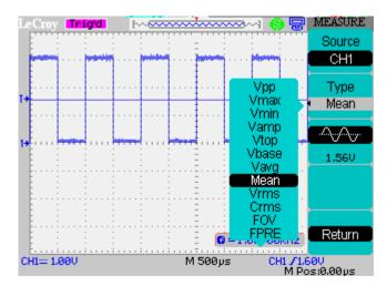
Press the front panel MEASURE button and your selected measurement is now shown (CH1 Vpp has been replaced by CH1 Mean).
