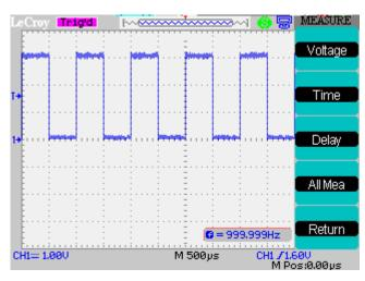
Now select the Voltage group, then Type and scroll to Mean. Leave the Source as CH1. In cases where more than one trace is in use the source can changed if required. Because we previously selected cursor mode as AUTO a cursor corresponding to the Mean value is displayed.
