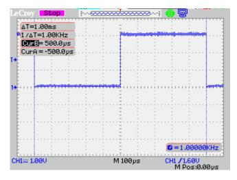
Press RUN/STOP to switch back to continuous triggering. Now select a timebase of 1us/div. In the CURSOR menu change Mode to Track. Now two cross-hair cursors are displayed. Select each cursor in turn and adjust to measure rising edge of the waveform.
