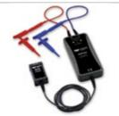
HVD Series high voltage differential probes permit measurements on power electronics circuits with floating voltages without reference to the ground, allowing the oscilloscope to be safely grounded. Excellent CMRR is provided at high frequencies and is combined with low inherent noise, high offset voltage capabilities, and high DC gain accuracy to make them an ideal choice for probing high voltage and floating control signals in single and three-phase power electronics designs.
