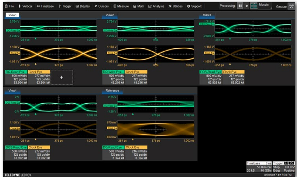
A complete system view is obtained by assigning measurement views to DQ-Read, DQ-Write, DQS-Read and DQS-Write. The reference view shows the DQ-Write eye while the system was using a different termination scheme.
