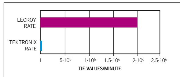
**TEKTRONIX-PROPOSED TEST 4:** Measurement of TIE (time-interval error) on a 622-Mbps data stream. (Note that we did not conduct test T3 because we ran out of time.)
