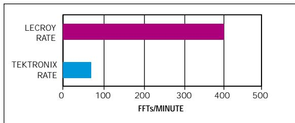
**LECROY-PROPOSED TEST 2:** Simple FFT measurement. (Note that we could not configure the TDS 6604 FFT record length to 100k samples.)
