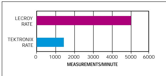
**LECROY-PROPOSED TEST 1A:** Simple 5.2-GHz sinusoid, with measurements of single-value-per-waveform, voltage-related parameters, such as peak-peak amplitude and rms value.
